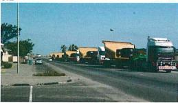
The above picture shows part of an abnormal shipment imported through Walvis Bay. The abnormal load comprised six disassembled 777D off highway dump trucks that were shipped from India and then transported by road to a local mine. The buckets and tyres in the above picture weigh approximately 30 tonnes each.
